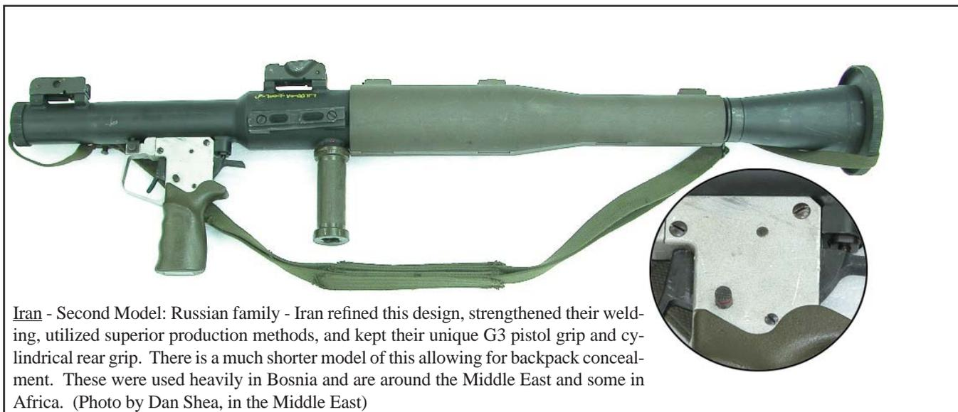
Iran - Second Model: Russian family - Iran refined this design, strengthened their welding, utilized superior production methods, and kept their unique G3 pistol grip and cylindrical rear grip. There is a much shorter model of this allowing for backpack concealment. These were used heavily in Bosnia and are around the Middle East and some in Africa. (Photo by Dan Shea, in the Middle East)
