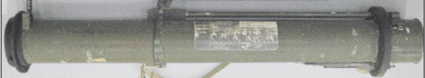
**RPG-26 AGLÉN** - RPG-26 is a disposable, non-telescoping Russian shoulder fired rocket launcher - again, not a recoilless. It is the direct replacement for the RPG-22 series, and the job it is for is taking out over 1,000 mm of concrete (about 3 feet) or 2,400 mm of log/earth bunker (over 7 feet). This is the same rocket as the RPG-22, with Graze features. The Thermobaric version is the RShG-2. (Photo by Dan Shea, taken in the Middle East)
